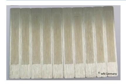
wfk F-PCD's ready for the assessment of the cleaning performance of WD's for surgical instruments: each PCD can be individually fixed at various positions of a tray and at different levels of a WD and cleaned together with real-life instruments, see picture below.
